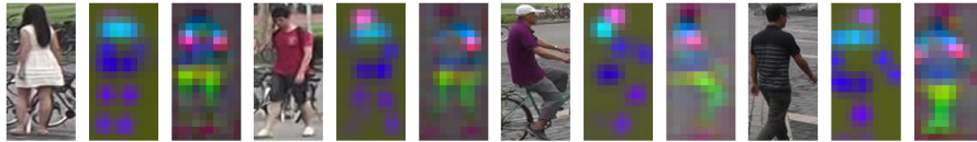
Fig. 5. Comparing the body part descriptors. For a given image (left), the conventional joint-based (center) and the proposed (right) descriptors are visualized. (Best viewed in color)
