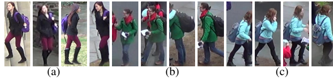
Fig. 1. (a, b) As a person appears in different poses/viewpoints in different cameras, and (c) human detections are imperfect, the corresponding body parts are usually not spatially aligned across the human detections, causing person re-identification to be challenging.
